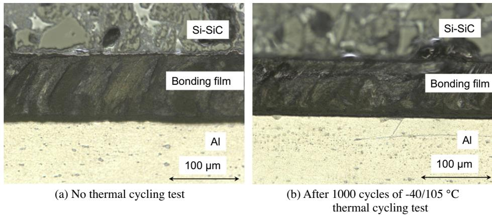
**Fig. 8.** Cross-sectional image of sample.
