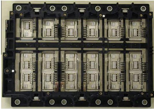
Fig. 1. Power semiconductor module.
